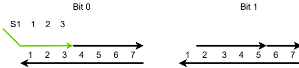
Fig. 8: One strand can be used to differentiate two bits
